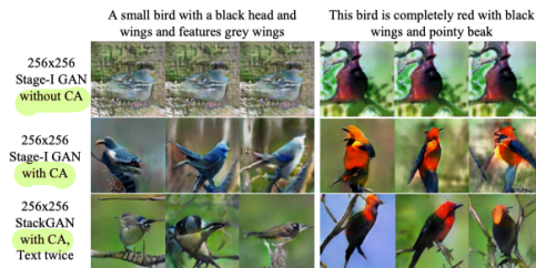
Figure 7. Conditioning Augmentation (CA) helps stabilize the training of conditional GAN and improves the diversity of the generated samples. (Row 1) without CA, Stage-I GAN fails to generate plausible 256×256 samples. Although different noise vector z is used for each column, the generated samples collapse to be the same for each input text description. (Row 2-3) with CA but fixing the noise vectors z , methods are still able to generate birds with different poses and viewpoints.
